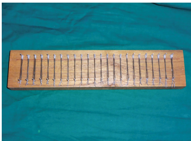
Fig. 1: Ligatures stretched on the model for the study
