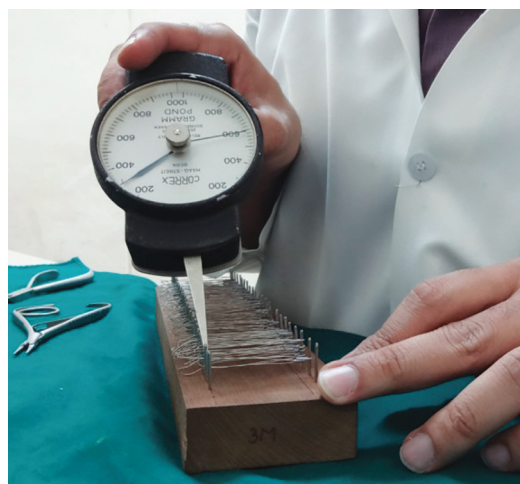
Fig. 2: Correx gauge being used for measuring force levels
